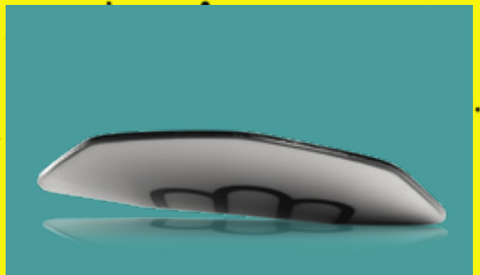
With a small amount of pressure and angle, the sidebases start to engage near the bindings, but the pressure remains constant along the contact edge.
