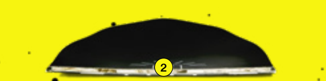
2. Increasing Uplift From Bindings To Widest Point Sidebase uplift gradually increases outside of the bindings to the contact points. The gradual rise creates smooth transition zones for turning and buttering, and the raised contact points make the board less susceptible to edge catch.
